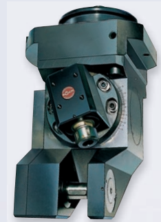
Milling unit with adjustable front head
